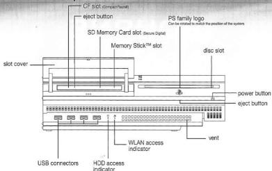
Set up the PLAYSTATION®3 system according to the instructions in its instruction manual. At start-up, the  $I\bigcirc$  indicator light will glow red to indicate that the PLAYSTATION®3 system is in Standby Mode. Press the  $I\bigcirc$ /RESET button and the  $I\bigcirc$  indicator light will turn green.
