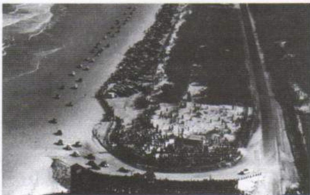
The original Daytona Beach race course, as seen from the air. The track was later lengthened from 3.2 miles to 4.1. After the first race, the chutes were graded with marl, a clay-like compound. (Daytona Racing Archives)
