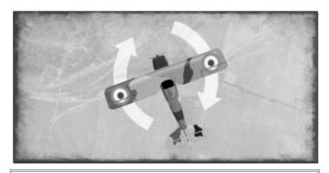
TO YAW LEFT, APPLY LEFT RUDDER; TO YAW RIGHT, APPLY RIGHT RUDDER.
